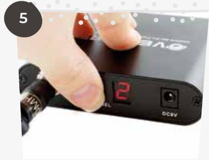
5 Assign a channel to the transmitter by pressing the channel button.
