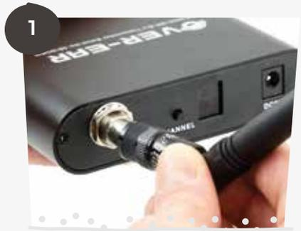
1 Fix the aerial provided onto the back of the transmitter.
