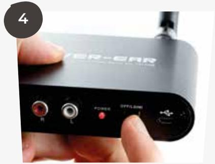
4 Switch the transmitter on by sliding the directly button to Hi.
