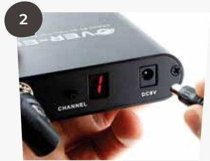
2 Plug the transmitter to the mains with the power cable provided.
